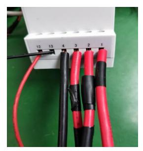
Port 5, 6, 7, 8, 9, 10 should be connected to the wires of CT secondary side.
