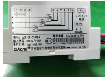
Port 1, 2, 3, 4 should be connected to A, B, C and N line of the three-phase grid for supplying the gird voltage to the meter.
