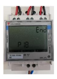
5. Scroll down up to the "end" option and press enter to exit programming menu.
