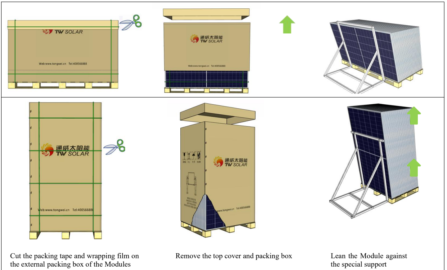
Figure 12 Schematic diagram of the unpacking procedure of the Module
