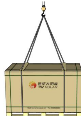
Figure 5 Schematic diagram of Module lifting
