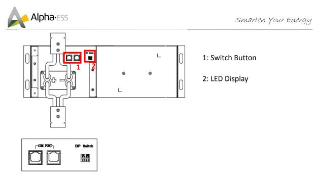
NOTE: if you use AlphaESS storage system please set the DIP switch 2 to "on" of the bottommost module .if you only use battery set the DIP switch 4 to "on" all the batteries.
