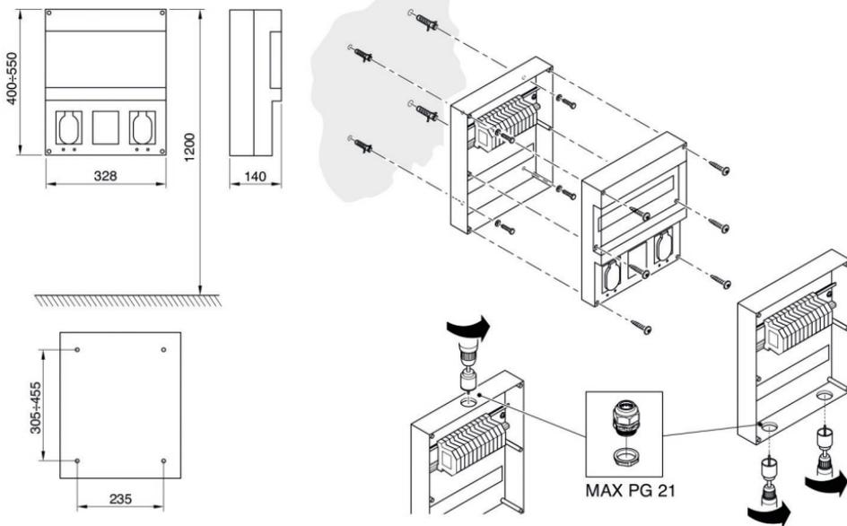
CABLAGGIO / WIRING / CÂBLAGE / CABLEADO
