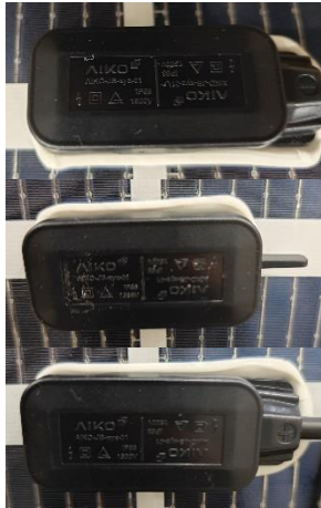
Fig. 10: detail view of closed junction box
