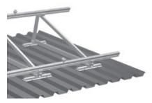
Installation with ballast on mounting rails
