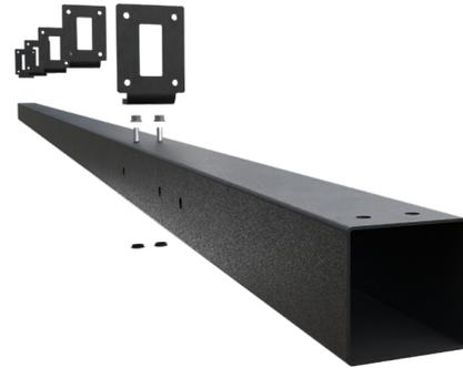
Attach two outer brackets (reversed to the others) to the rafter. Two M12x35 cylinder head screws, four washers and two M12 nuts are needed per angle. The screws are inserted from below.
