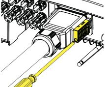
▲ ATTENTION – The AC quick fit connector must not be subject to tensile forces (examples: do not connect weights to the AC cable, do not leave excess cable windings hanging, etc).
