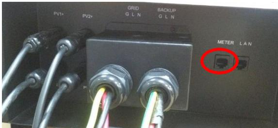
Plug the free end of the RS485 cable into the slot on the backside of the cabinet.
