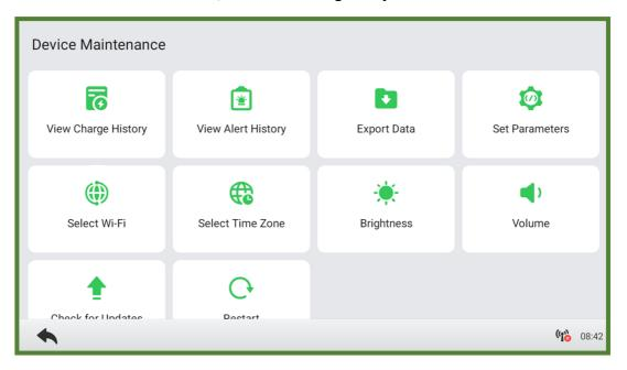
6. In some cases where the MaxiCharger uses a third party platform instead of Autel cloud platform, you may need to manually set the parameters by tapping **Set Parameters** on the Device Maintenance Screen.
