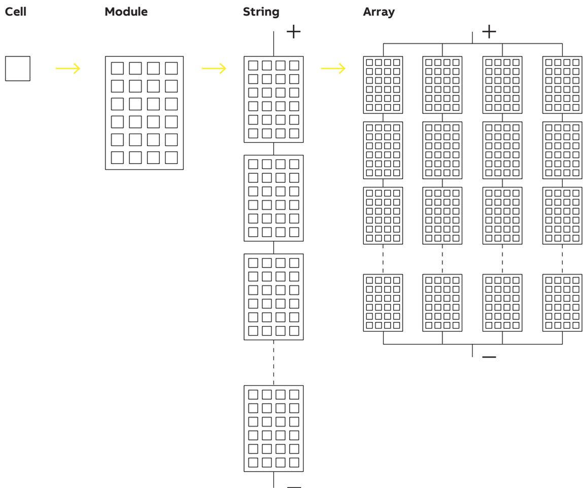
The current of each array must fall within the rating value limits of the inverter.
