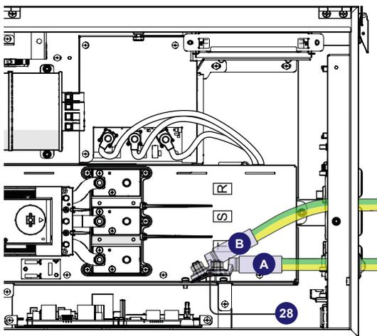
**⚠ ATTENTION** – Depending on the version of the AC panel installed on the inverter it will be necessary to use a different protection earth connection point in order to avoid mechanical stress due to cable bending: in
