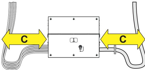
**NOTE** – In case of manual installation, using handles (04), consider a free side space to lift the inverter of **60 cm** minimum.
