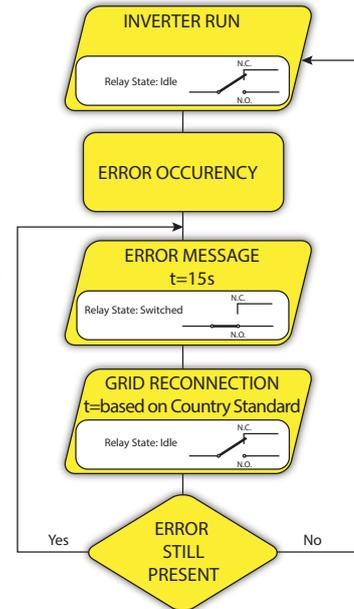
In the presence of W003, W004, W005, W006, W007 signalling, the alarm contact switches and then reset itself at the end of the alarm signal. This means that during the absence of grid voltage (display message “Missing Grid”) the alarm contact remains in its resting position.
