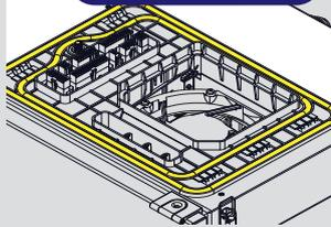
Any damage on the gaskets could cause serious fault to the unit and will lead to the invalidation of the warranty.
