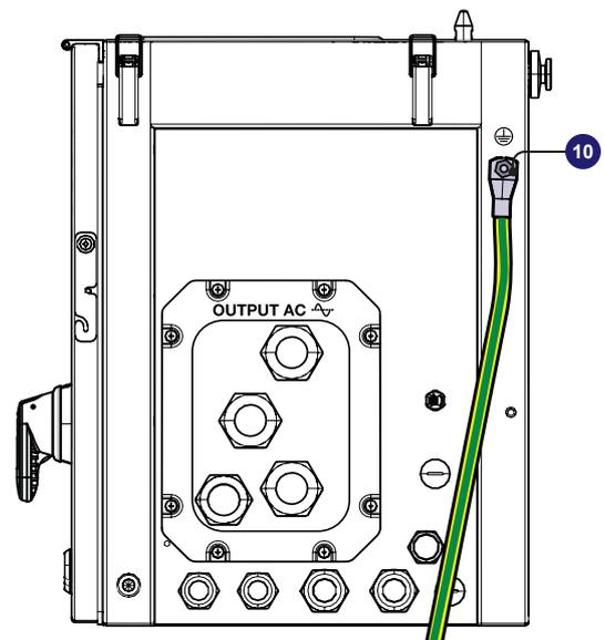
**⚠ ATTENTION** – The cable lug must be installed with a tightening torque of 15.2 Nm.
