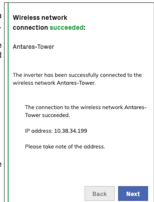
**NOTE** – The IP address assigned may vary for reasons related to the wireless router setup (for example, a very brief DHCP lease time). If verification of the address is required, it is usually possible to obtain the client list (and the corresponding IP addresses) from the wireless router administration panel.
