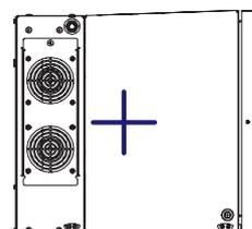
Center of gravity (wiring box)
