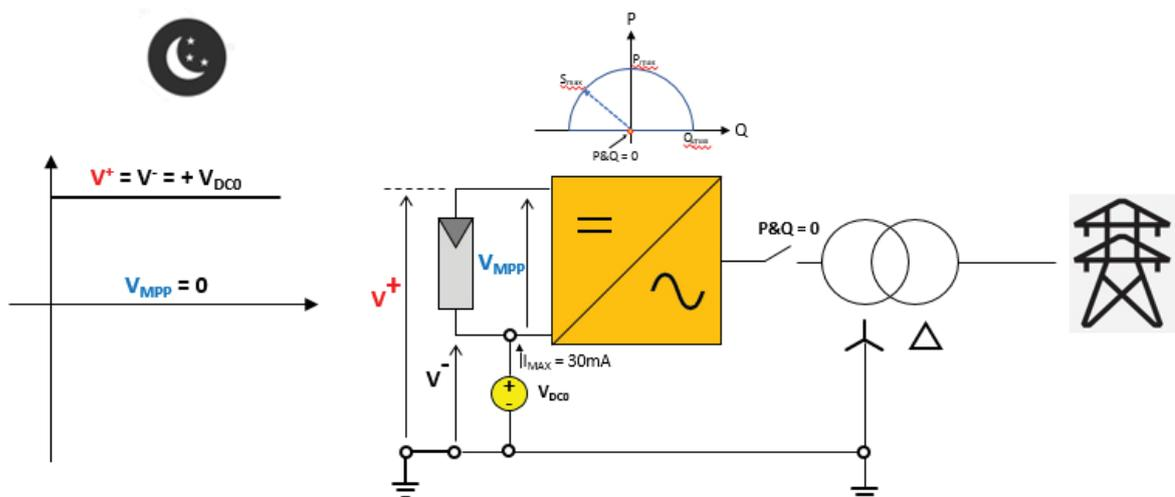
In the figure PVS-175's array terminal voltages with respect to ground during night-time operation of the Anti-PID board, inverter is off-line
