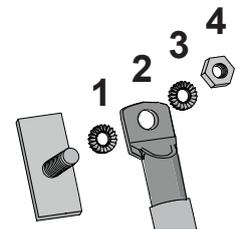
**⚠ ATTENTION** – The cable lug must be installed with a tightening torque of 3Nm (2.2 ft-lb).
