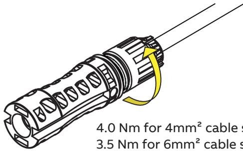
4.0 Nm for 4mm<sup>2</sup> cable section
