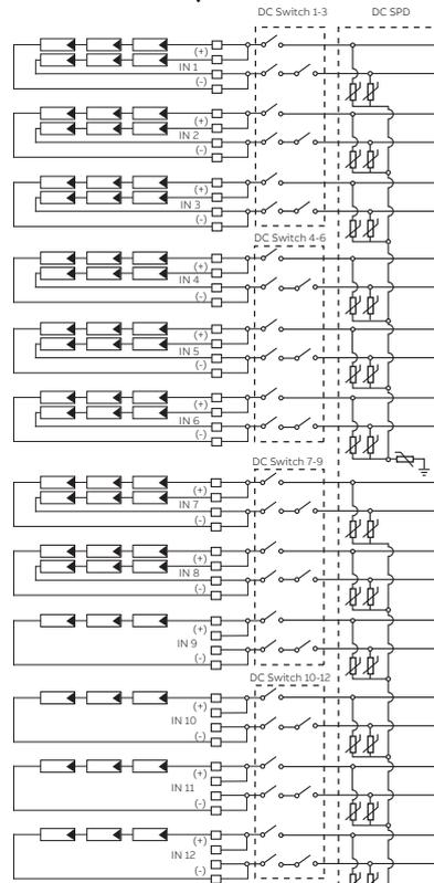
**$N_s < 12$  (11 in this example):** connect one string each from MPP1 to MPP11 or from MPP2 to MPP12.
