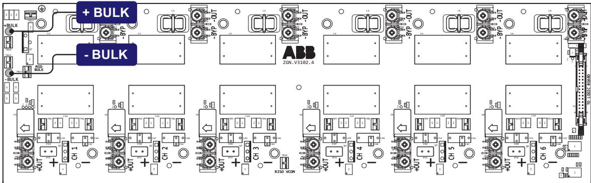
**15. Voltage absence test on mid bulk point (Power Module)**
