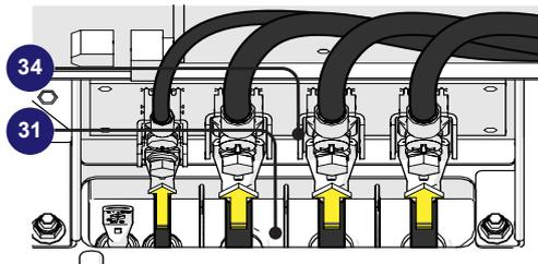
**⚠ ATTENTION** – In case of a wrong phase sequence the inverter will not connect to the grid and it will provide an error state.
