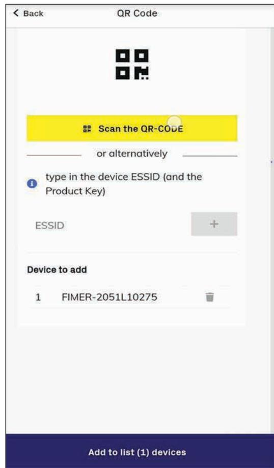
**NOTE** – Both QR code and Product key are provided on the Communication identification label applied onto each inverter or applied on the plant documentation (if this has been done during installation).
