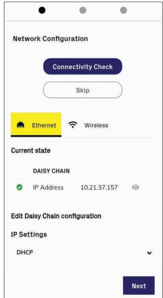
**NOTE** – When the networking configuration is concluded, it is possible to test the inverter connectivity to internet and Aurora Vision cloud services.
