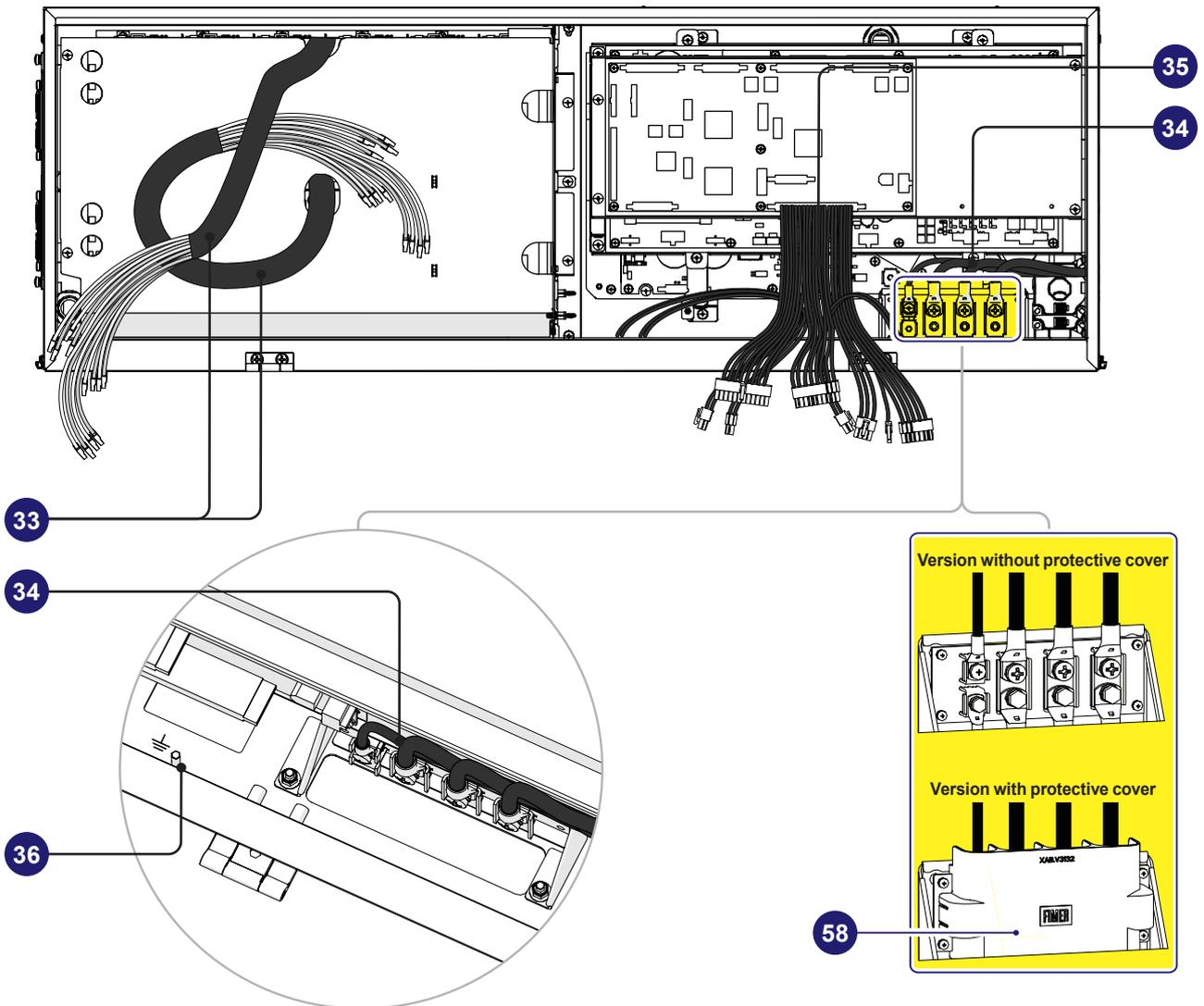
PVS-175-TL - Wiring box Internal view
