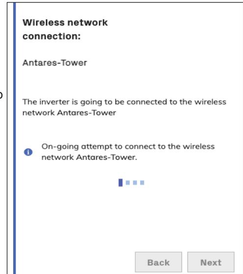
Once the inverter is connected to the wireless network, a new message will confirm that the connection is acquired.
