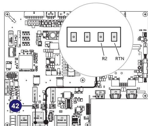
The external switch used for Remote ON/OFF should be rated for DC low voltage, low current application (the minimum switching current capability should be 1mA or lower).
