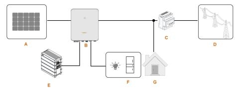
figure 2-3 PV Energy Storage System (PV ESS)
