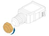
step 2 **(Optional)** Remove the inner sealing ring if the cable diameter is between 19 mm ~ 25 mm. Otherwise skip this step.
