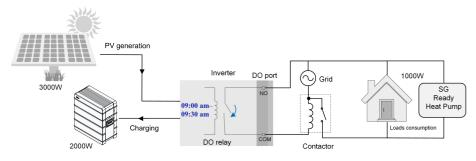
figure 8-38 DO Operation in Intelligent Mode
