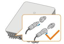
step 2 Ensure that the connectors are securely in place.
