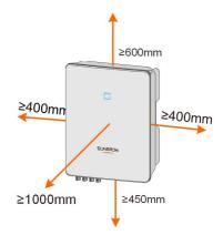
In case of multiple inverters, reserve specific clearance between the inverters.
