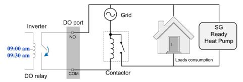
figure 8-36 DO Operation in Timing Mode
