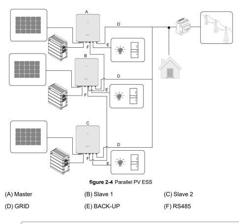
Only the hybrid GRID terminals can be connected in parallel, the BACK-UP terminals and the battery terminals cannot be connected together. Each hybrid must have its own BACK-UP loads. The Backup loads of each inverter should not exceed its nominal power.
