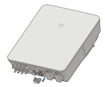
step 2 Insert the COM connector into **COM** terminal on the bottom of the inverter until there is an audible click.
