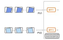
For SH10RT/SH10RT-20, each pair of PV terminals is corresponding to an independent PV string. PV input PV1 connect to MPPT1 and PV2, PV3 connect to MPPT2. For the best use of PV power, PV2 and PV3 should be the same in PV string structure, including the type, number, tilt, and orientation of the PV modules.
