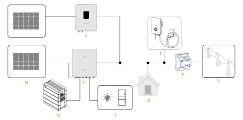
figure 2-11 Retrofitted PV Storage and EV-Charger System
