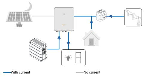
During night, when the battery is empty, it will enter into standby mode. In this case, the grid will supply all power for loads.
