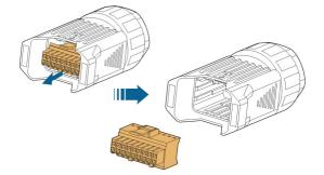
step 3 Remove the seal and lead the cable through the cable gland.
