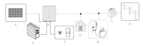
figure 2-8 PV Storage and EV-Charger System
