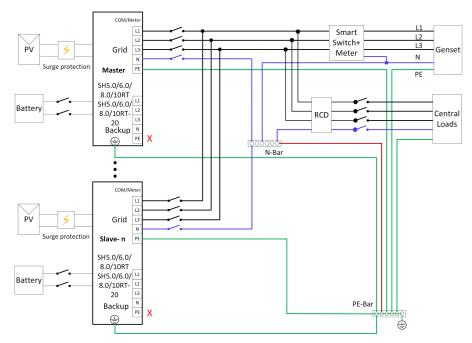
figure 2-6 Wiring diagram for Australia and New Zealand
