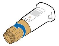
step 4 Thread the network cable through the swivel nut and gasket. Afterwards, route the cable into the opening of the sealing. Finally, insert the cable through the housing.
