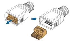
step 4 Thread the AC cable of appropriate length through the swivel nut and the housing.
