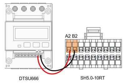
• For SH5.0–10RT-20, please connect Pin A on the smart energy meter DTSU666–20 to Pin A2 on the inverter and Pin B on the meter to Pin B2 on the inverter.
