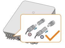
step 2 Check for polarity correctness.
