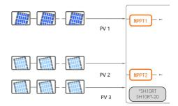
For SH10RT/SH10RT-20, if two PV strings are paralleled externally, the paralleled strings can be connected to PV2 or PV3 only, and the other one cannot be used to connect other PV strings.
