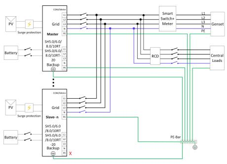
figure 2-7 Wiring diagram for other regions \*
