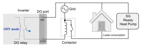
figure 8-37 DO Operation in Switch Mode
