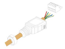
step 5 Strip 80 mm ~ 90 mm of the cable jacked and 12 mm of the wire insulation.
