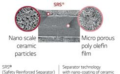
with nano-coating of ceramic particles
